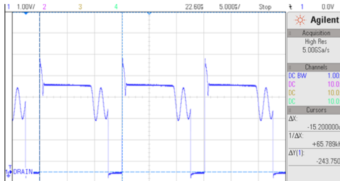
Fig:7 Vds at full load by using DF probe 1:100 at 230V AC
